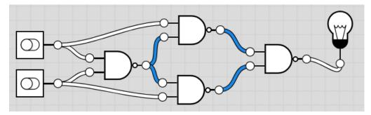
The XOR gate is the hardest to understand. It is composed of four NAND gates.
